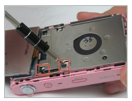
Once the camera is open, remove the two internal screws using a Phillips 000 screwdriver.
