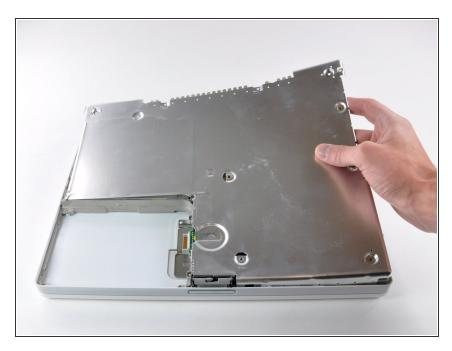
• Lift the bottom shield off.
