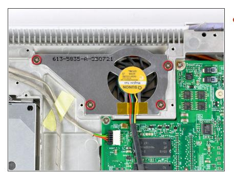
Remove the 4 Phillips screws securing the fan to the metal framework.
