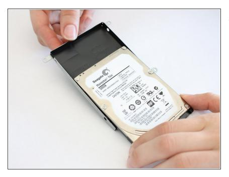
Slide the hard drive out of the bracket.
