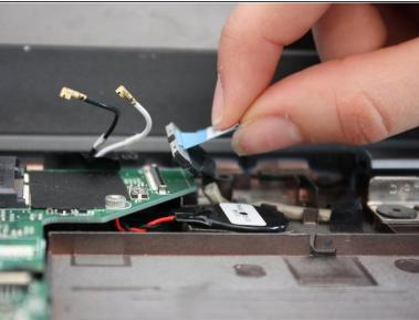
Gently pull the the blue ribbon upwards to disconnect the computer from the motherboard.
