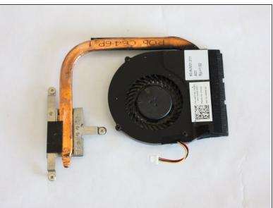
Remove the fan from the motherboard by lifting upwards.
