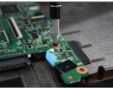
Using a J0 tipped screwdriver remove the 6 mm Phillips head screw located at the center of the laptop on the motherboard.
