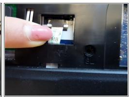
Disconnect the two blue and white ribbons by applying pressure downward and pushing them out of their sockets.
