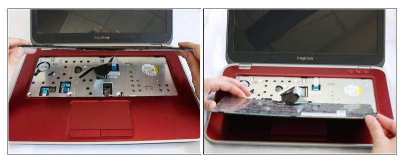
• Flip the keyboard over onto the palm-rest assembly.
