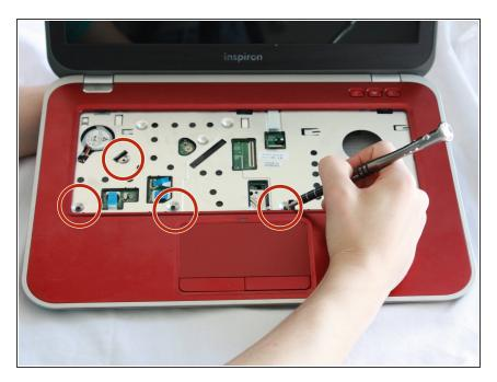
Use J0 Bit screwdriver to remove all four 6 mm Phillips screws.
