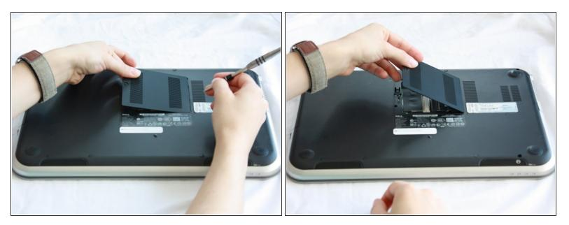
• Lightly lift the RAM cover up and at an angle, away from the computer.
