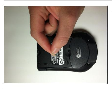
Open a standard paper clip and insert into the end into the hole for the button. Gently press the button.
