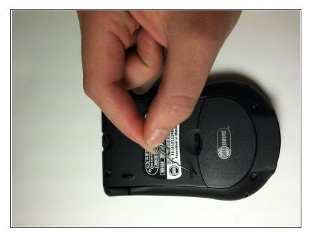
Locate the reset button on the back rear cover labeled "reset" just above the battery cover.
