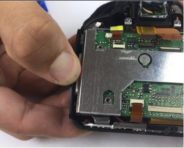
Gently pull out the side wall of the camera so that the motherboard comes out easier.
