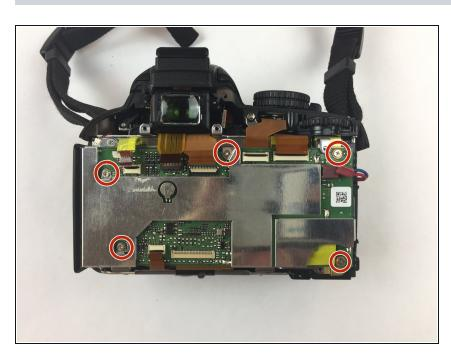
Use a Philips #00 Screwdriver to remove the five 3 mm screws marked in the image.
