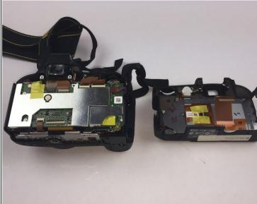
• Starting from the top, gently lift the back panel of the camera off. Slowly separate the back panel from the main body of the camera.
