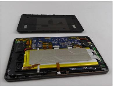
Once the back panel has been pried away from the bottom and sides of the Neo3DO, lift the back panel up and away from the tablet.
