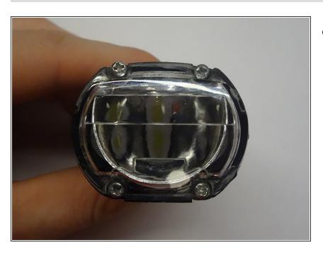
Remove the four screws that attach the lens to the metal cooler of the LED
