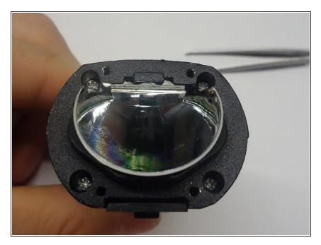
This reveals the four screws holding the plastic back cover to the metal central chassis. Remove them as well
