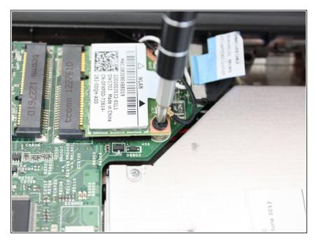
Using a J0 tipped screwdriver, remove the 4 mm Phillips head screw.
