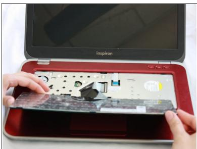
Flip the keyboard over onto the palm-rest assembly.
