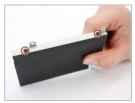
Using a J0 bit tipped screwdriver, remove the four 3 mm black screws on both sides of the hard drive bracket.
