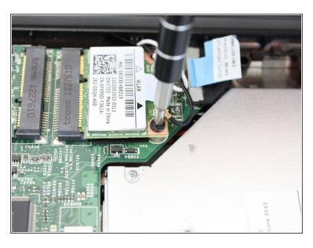
Using a J0 tipped screwdriver, remove the 4 mm Phillips head screw.
