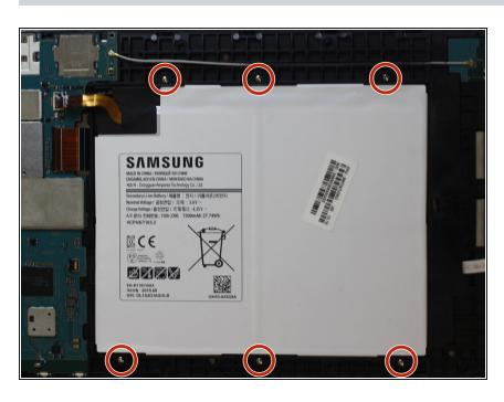
There are a total of six 3mm PH000 screws holding the battery in place.
