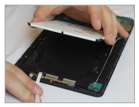
After thoroughly detaching the battery from the adhesive glue, pull the battery up and out of its housing.
