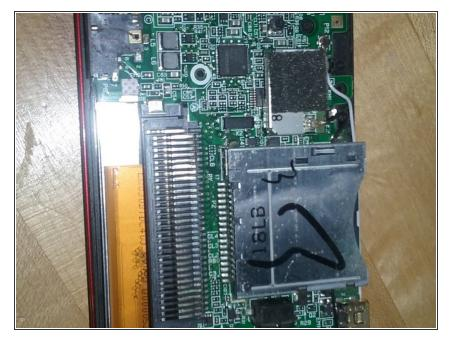
Your first step would be to unscrew all all screws on the back and take the case off. You take the case off by placing a spudger on the line edges, and then place it inward, forcing it to separate the two parts.
