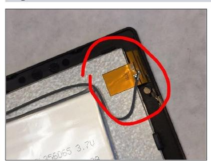
The battery is attached in two different ways; one wire is attached to the screen to support the screen's background led lights.
