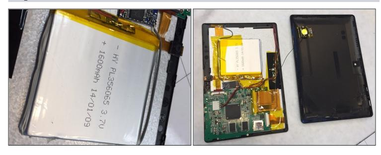
• The battery will appear as pictured. Separate the back case from the device. Avoid damaging the wire that connects the speakers between the two halves of the case.
