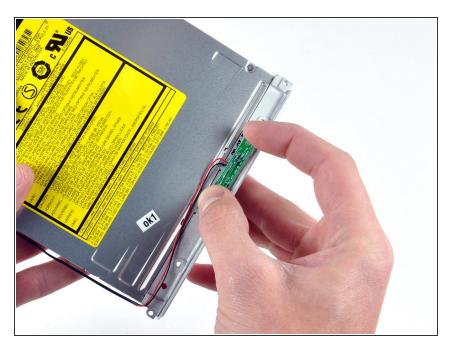
Peel the reed switch board from the optical drive and set it aside.
