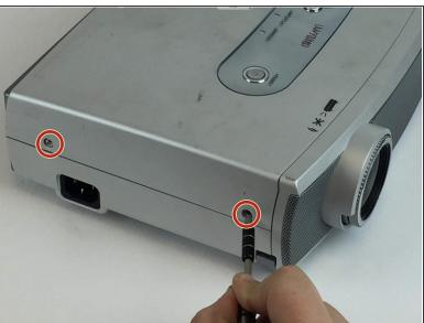
• Remove the 4 exterior 9mm Phillips #0 screws. They are located on the sides of the projector.
