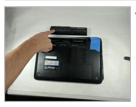
Locate and remove the battery from device
