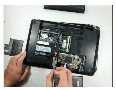
Remove the screw that locks the CD drive in place
