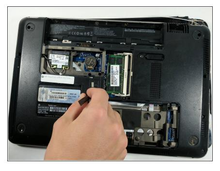
Push on the rear end of the CD drive with a small non-metallic item to free it from the case
