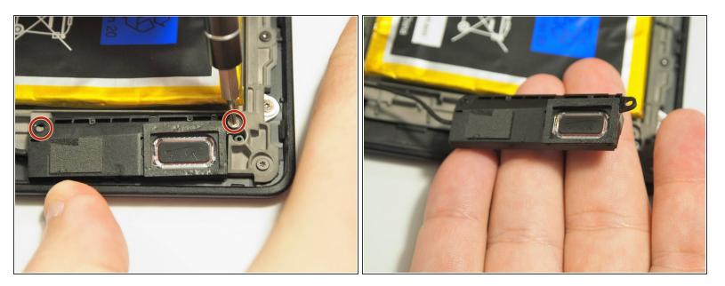
• Remove (2) 3mm T4 Torx screws from the bottom speaker.
