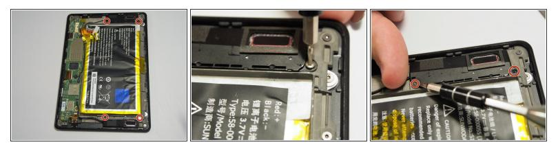
There are (4) 3mm T4 Torx screws between both speakers (two each). Remove the ones necessary for whichever speaker needs to be replaced.
