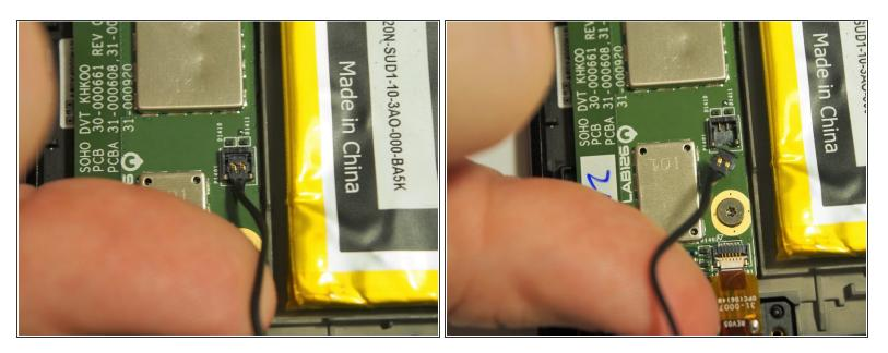
Same as Step 3, after the screws are removed, follow the wire to where it connects and pull up gently until it disconnects.
