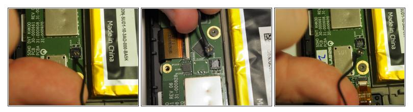
After the screws are removed, locate the wire, follow it to where it connects to the main device, and pull up gently until it disconnects.
