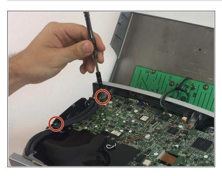
Remove the two 7mm Phillips #0 screws that attach the fan to the motherboard of the projector.
