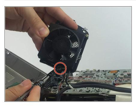
Remove the 7mm Phillips #0 screw that fastens the black ground wire connected to the fan and the projector.
