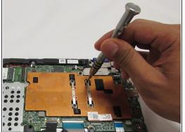
• Use the phillips screwdriver with the PH0 to loosen the 4 screws and remove the orange plate.
