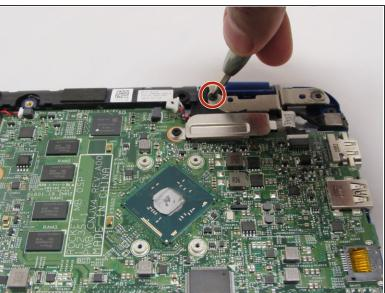
• Use the phillips screwdriver with the PH00 head to unscrew the one 3mm screw. Then, remove the bracket.
