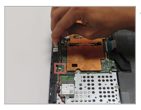
Use the tweezers to remove the CMOS Cable.
