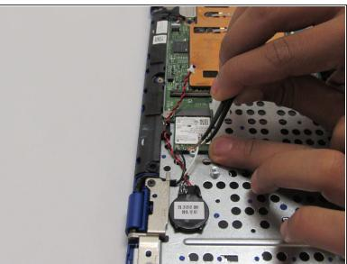
Using the tweezers, pull the white and black wires off of the WiFi Chip.
