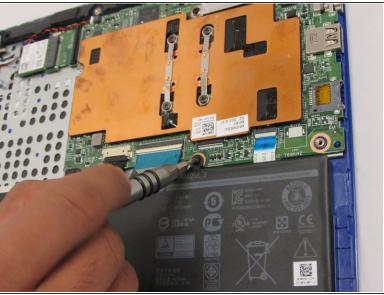
Use a Phillips screwdriver to unscrew the three 4 mm screws securing the battery.
