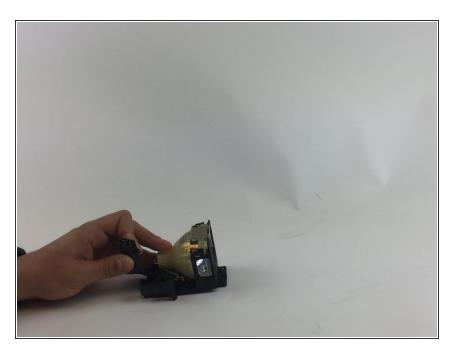
Pull the wire tubing out of the plastic holder.
