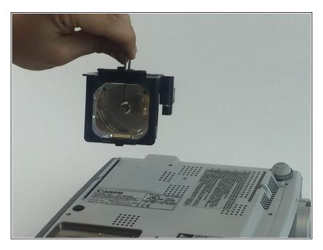
You may replace the entire housing unit or replace the bulb itself once you remove it from the housing unit.
