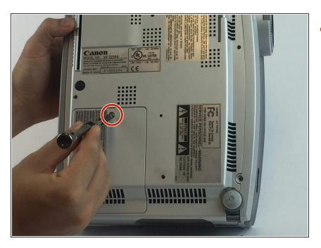
Unscrew the 9mm Phillips #0 screw and remove the panel.
