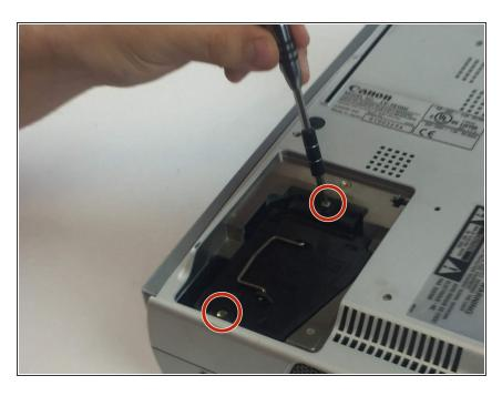
Unscrew the two 7mm Phillips #0 screws that attach the bulb to the mainframe of the projector.
