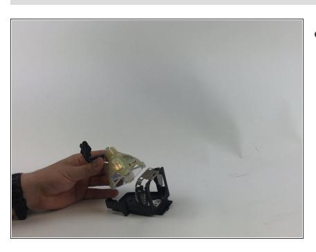
Pull the bulb out of the casing.
