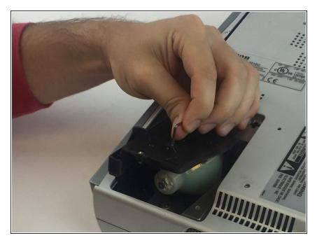
Remove the bulb housing by gently pulling on the small silver handle located on top of the bulb housing.
