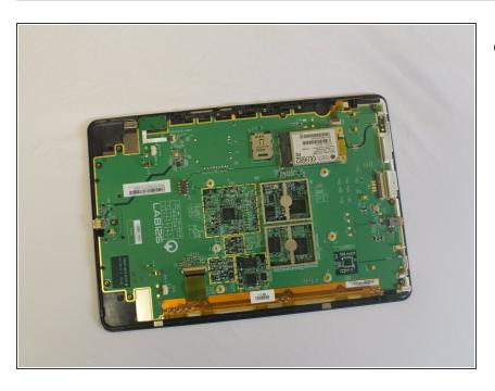
Remove the motherboard from the display assembly.
