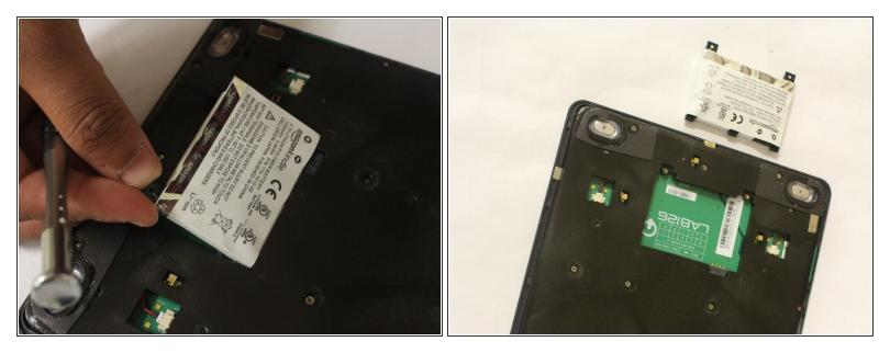
Take the battery off once the screws have been removed.
