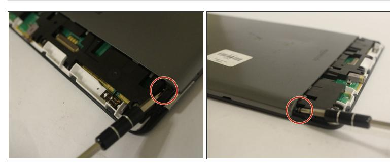
Once the small plastic piece is removed you will need to locate two 40mm screws on both corners
