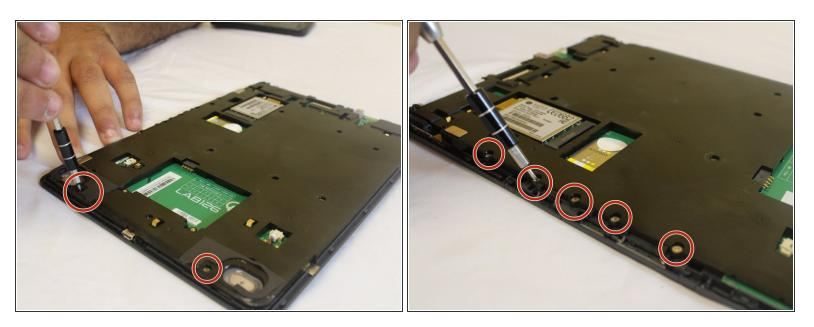
Unscrew the 30 mm screws using a Phillips #000 screwdriver as shown in the picture.
