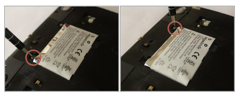
Locate the two 30mm screws securing the battery on the bottom of the Kindle DX. Use the PH00
