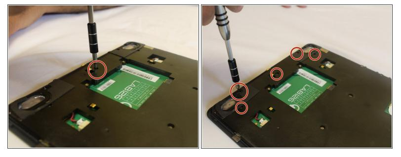
Unscrew the 30 mm screws using a Phillips #000 screwdriver as demonstrated in the picture.
