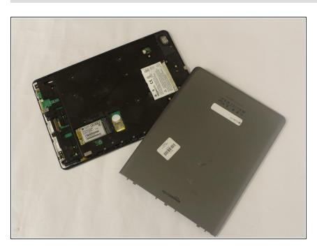
Once the piece removed, locate the battery.
