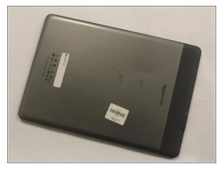
Take your Kindle and place it screen side down in order to open it from the back. Use the opening tool from the ifixit tool kit and insert it between the metal casing and plastic top piece.
