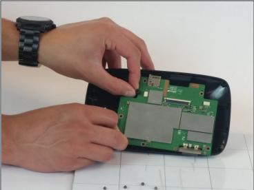
• Disconnect the battery and speaker ribbon cables from the motherboard.
