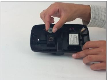
• Use a spudger to remove the speaker from back case.
