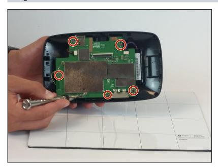
Remove all six screws from the motherboard with a Philips #000 screwdriver.
