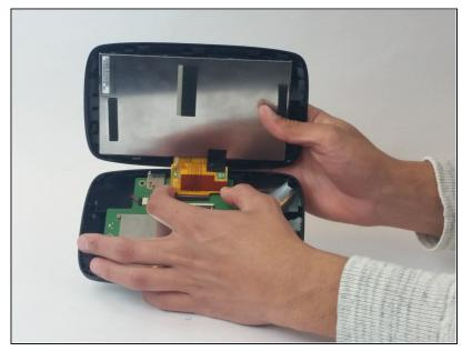
Disconnect the screen from the motherboard by removing the yellow ribbon connector from the socket.
