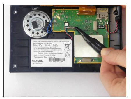
Using the angled tweezers, grip the red, black, and green wires connecting the battery to the motherboard, then gently lift away from the motherboard.
