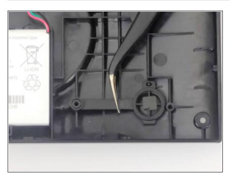
Using tweezers, lift the button out of its socket.
