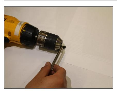
Insert the Allen wrench into the chuck jaws and tighten the jaws down on the wrench.
