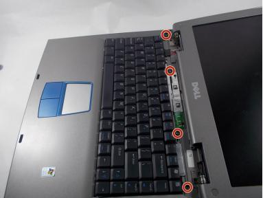
Remove the four 3mm Phillips #0 screws securing the keyboard.
