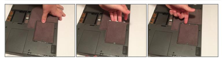
Slide the cover towards the screw, and then lift the cover upwards.
