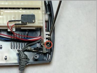
Remove the wire holder. This is a small screwed in piece of plastic which holds the wires in place.
