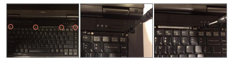
With a Phillips #1 screwdriver, unscrew the four-six mm screws that were hidden under the plastic piece you removed.
