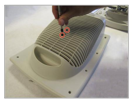
Remove two Phillips #2 12mm screws from housing
