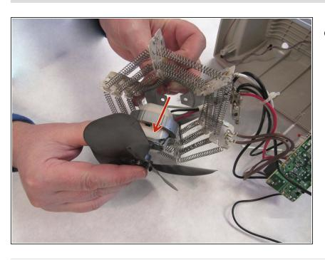
Separate fan assembly from heating coil
