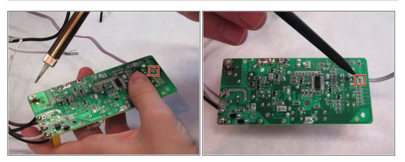
Desolder the WHITE connector (attached to the GRAY wire coming of the thermostat) from the "NTC101" point.
