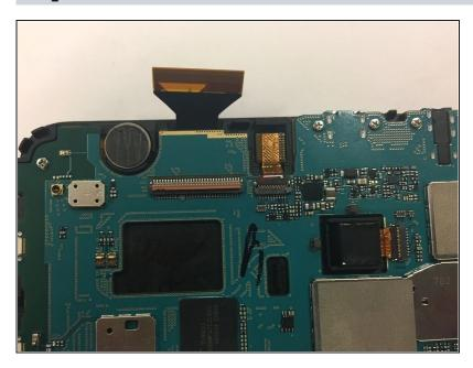
Once you've undone the connector lock, use a pair of tweezers to pull the cable front its housing.
