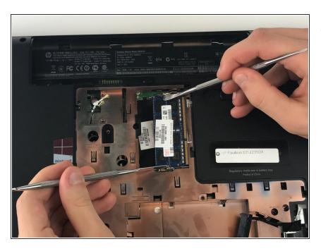
Using either your fingers or two metal tools, push outwards on the two prongs until the RAM card pops out.
