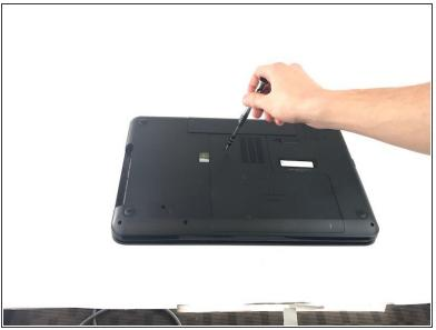
Loosen the 7.25mm screw on the bottom of the laptop holding the "L" shaped cover down.
