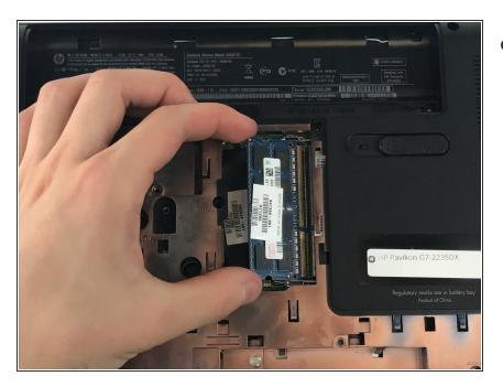
The RAM card can now be pulled out at a slight angle.
