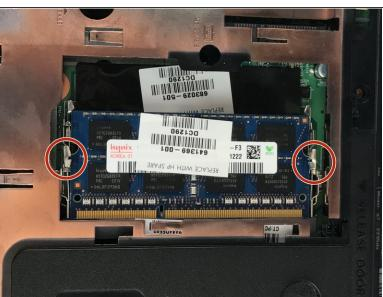
Locate the RAM card and the two prongs holding it in place.
