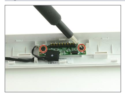
Use a Phillips #00 screwdriver to remove the two 4.3mm screws holding the circuit board in place.
