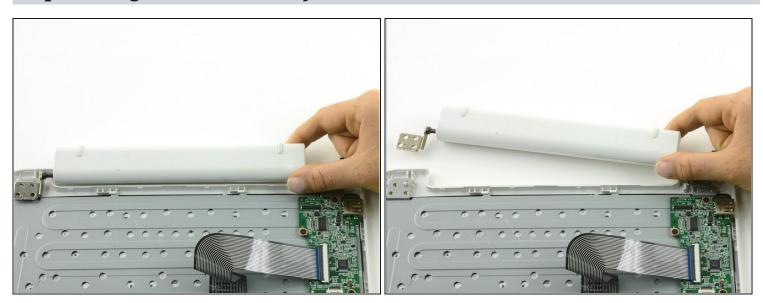
• Lift the hinge away from the device.
