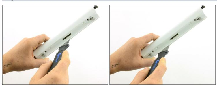
• Slide a Jimmy or other prying tool along the seam of the hinge to pry the casing apart.
