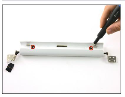
Use a Phillips #00 screwdriver to unscrew the two 6.5mm screws.
