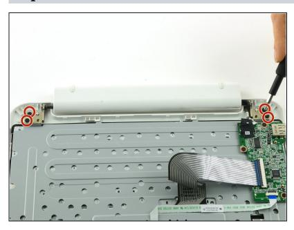
• Use a Phillips #00 screwdriver to unscrew the four 6.4mm screws on the hinge mounts.
