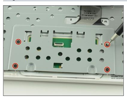
Use a Phillips #00 screwdriver to unscrew the four 6.4mm screws holding the touchpad in place.
