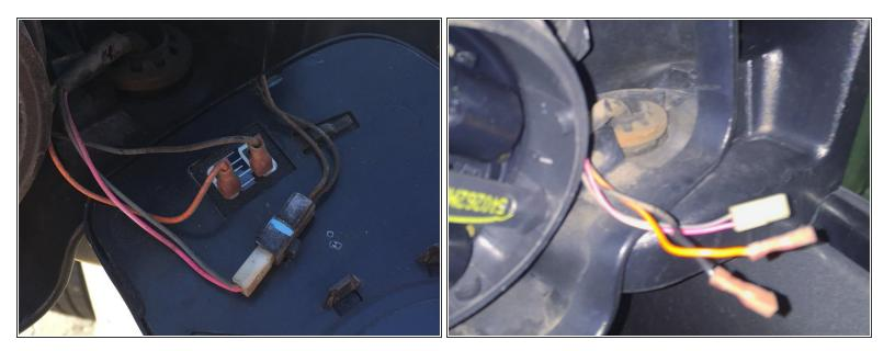
Unclip all three wires and remove the old mirror from the module.
