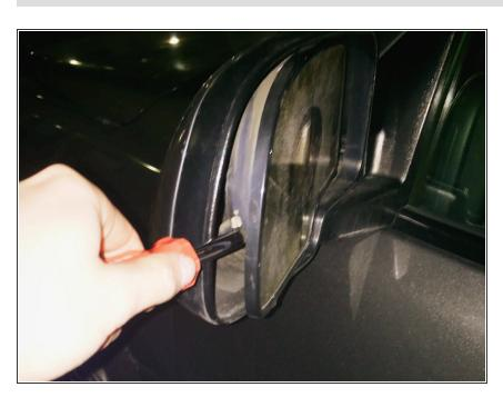
Insert the screwdriver on the left side of the mirror and apply force to release.
