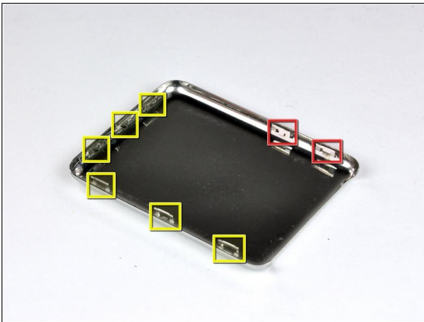
**i** The rear panel is secured to the front case by eight clips permanently attached to the rear
