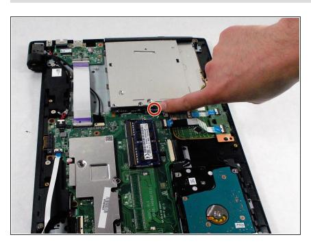
Unscrew one 3.0 mm screw from the disk drive using a #1 Phillips screwdriver.
