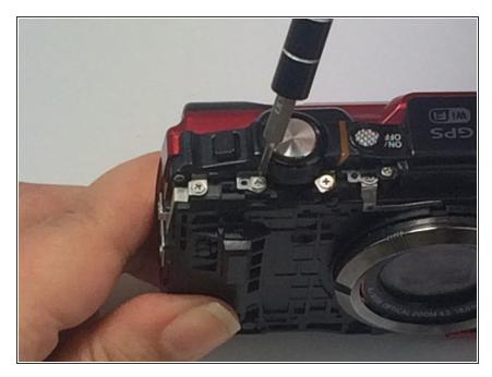
Use the PH000 screwdriver to remove the 3mm screw shown on the picture.
