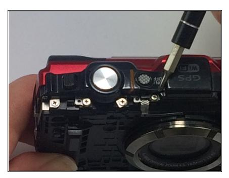
Use the PH000 screwdriver to remove the 4mm located below the ON/OFF button.
