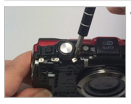
Using the PH000, remove the 3mm screw shown on the picture.
