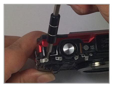
Use the PH000 screwdriver to remove the 5 mm screw located on the top left side of the device.
