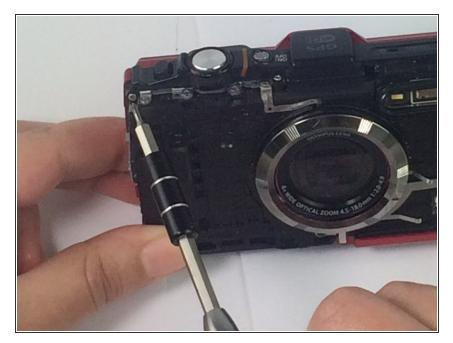
Use the PH000 to remove the 7mm screw on the upper right corner of the device.
