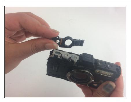
Using your hand, remove the plastic button holder containing the shutter and ON/OFF buttons. The buttons and metal springs under it are now unlocked.
