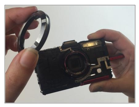
Twist the ring around the camera lens and pull it out.
