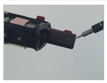
Use the PH000 screwdriver to remove both 2mm screws holding the gasket of the HDMI port door. Remove the rubber gasket.
