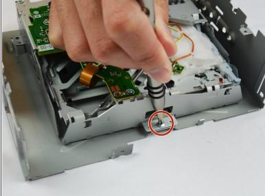
Use the Phillips #0 Screwdriver to remove the three screws.
