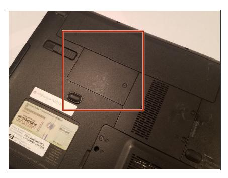
Begin by locating the smallest panel with one screw attaching it to the laptop computer.
