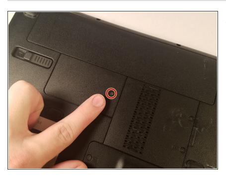
Remove the one screw holding the panel down, and the WiFi receiver will be revealed.
