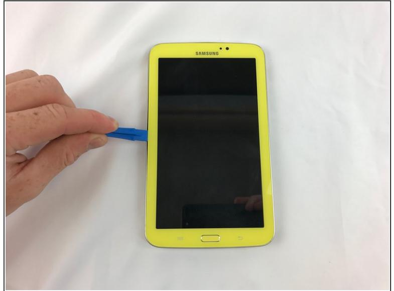
**⚠ Before disassembling your phone, discharge the battery below 25%. A charged lithium-ion battery can catch fire and/or explode if accidentally punctured.**
