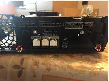
Remove the three remaining screws on the lower plastic of the device.
