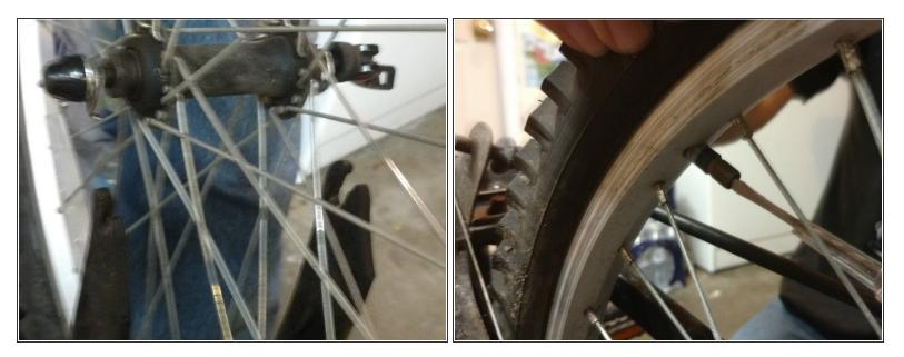
• Once Unscrewed the wheel will slide off (You might need to lower air pressure in the tires to allow them through the break pads). Put the wheel to the side.
