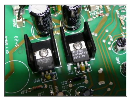
The left is a PNP transistor (TIP32C) and the right is a 15V linear voltage regulator (LM7815), but that is not the reason I took the picture. Look at the middle pins on the packages, they have a little tube around the legs. I am not sure, but I guess it is to prevent a short if something metallic fell near the legs.
