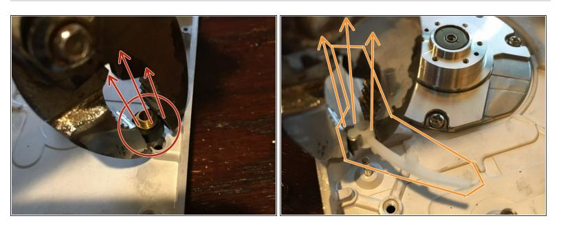
Use a pair of pliers to remove the brass/rubber standoff (circled in red in the first picture) and the plastic bar ("circled" in orange in the second picture) from the aluminum drive body. Pull hard and pull up.
