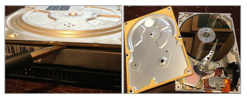
Now, pull off the drive cover. Pry where a yellow strip of sealing rubber appears. Pull off the drive's cover, and then move on.
