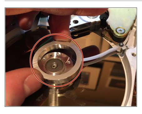
Now, pull off the aluminum spacer (circled in red) in between the two platters (see the next step for a picture of this). We can't remove the second disk just yet, so let's move on for now.
