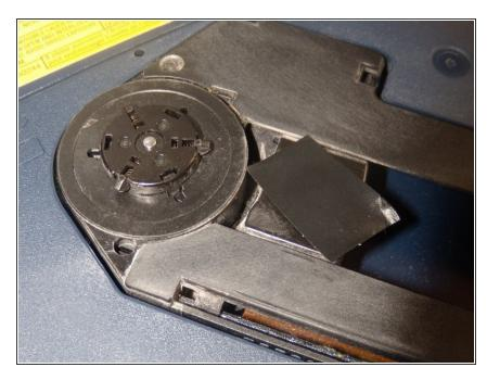
Place a small piece of tape over the lens. You need to use something with minimal stickiness. I used electrical tape. This is to protect the lens when you do the sanding.
