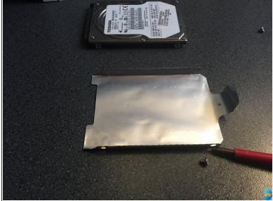
Remove the 4 screws from the hard drive.
